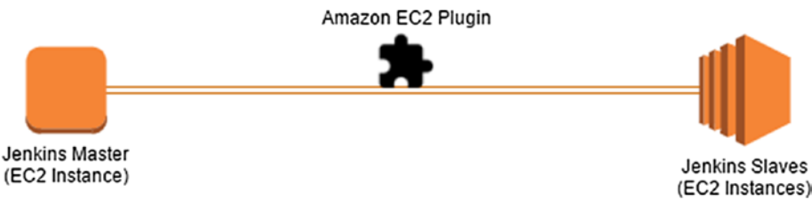
Figure 4-9. Scalable Jenkins Slave cluster using EC2 Instances
